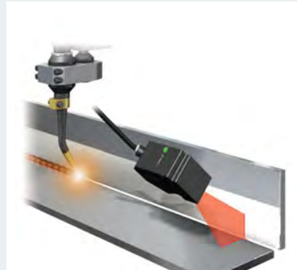
Position feedback in an automated welding operation
