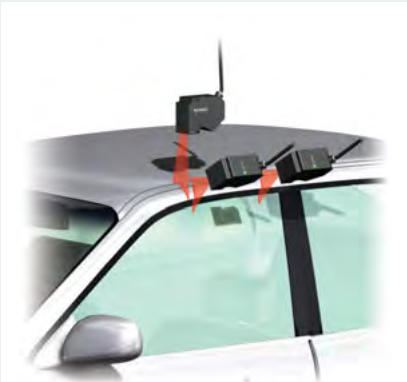
Checking the assembly accuracy of an auto body
