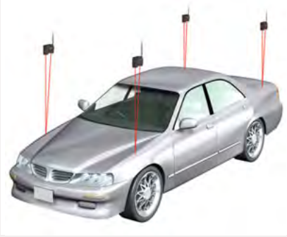
Measuring height of an air suspension vehicle
