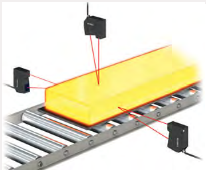
Measuring the width/bulging of slab material
