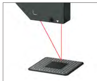
Measuring the shape of BGA
