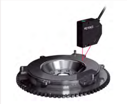
Measuring the surface runout of a flywheel
