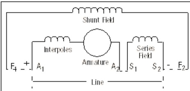
Stabilized shunt motors utilize a field winding in series with the armature in addition to the shunt field to obtain a compromise in performance between a series and shunt type motor. This type offers a combination of good starting torque and feed stability.
