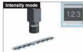
Intensity mode Differentiation of the correct/incorrect sides of a chip component Differentiates correct/incorrect sides of a chip based on the difference in brightness
