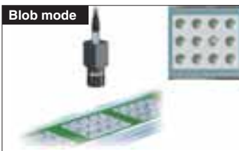
Blob mode Counting the number of tablets Counts the number of properly shaped tablets
