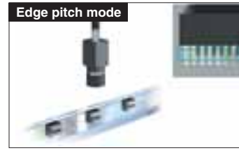
Edge pitch mode Inspection of the lead pitch of a connector Measures the center pitch of connector pins
