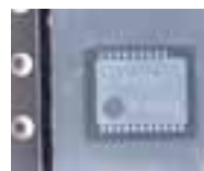
With monochrome camera and red light clear contrast is created through the film.
