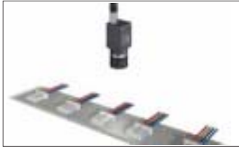
Checking correct cable assembly
