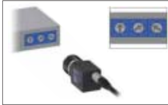
Inspection of trimmer switch position
