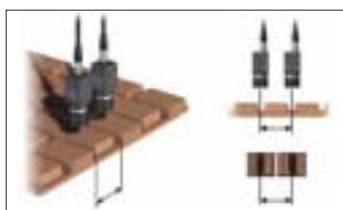
Pitch measurement of construction boards
